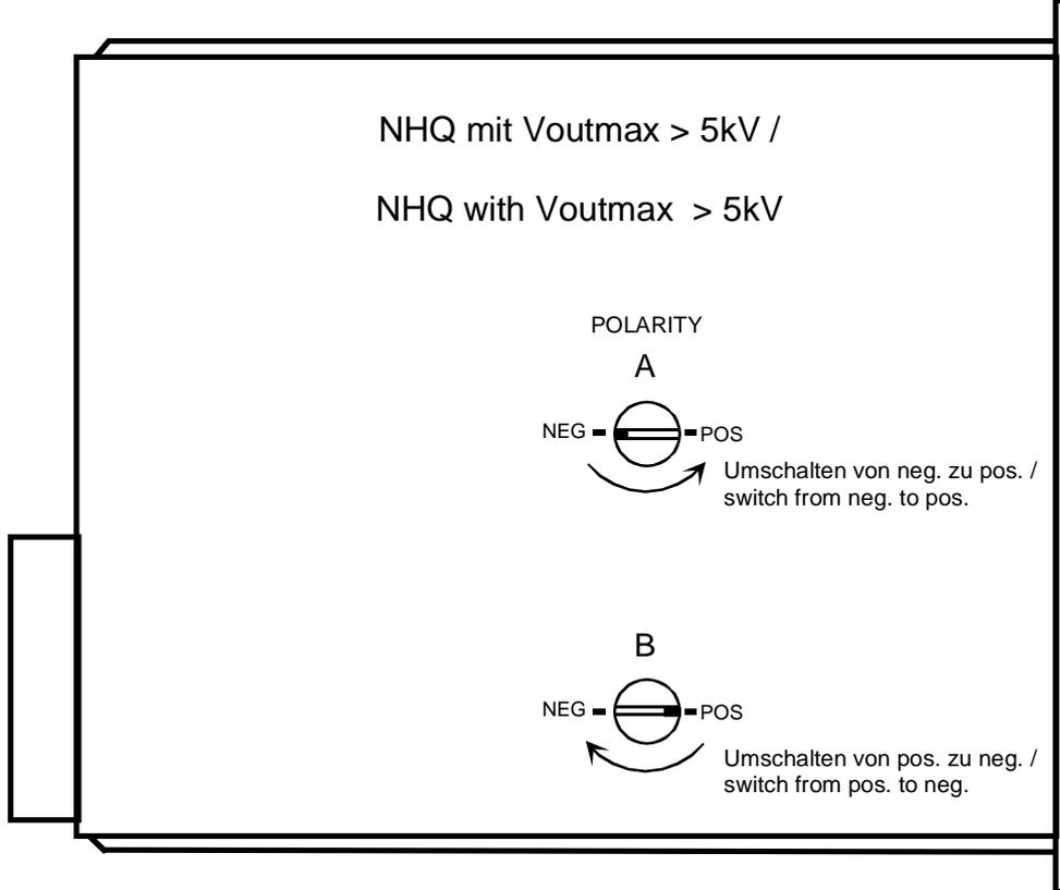
**Appendix B:** NHQ side cover, Polarity rotary switch
