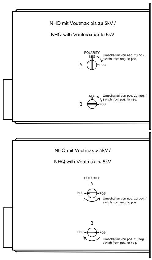
**Appendix B:** NHQ side cover, Polarity rotary switch
