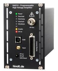
The HA51U series is a family of single channel, bipolar, unipolar and unsymmetrical high voltage amplifiers. They feature high speed, high precision and high stability as well as very low ripple and noise. They are designed to drive capacitive and resistive loads. High peak output current facilitates easy driving of capacitive loads.
