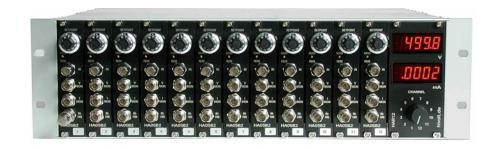
The high voltage amplifier HAR12A is a 19'' rack-mountable unit of 3HU. Twelve channels provide output voltages in the range of -500V to +500V at load current of  $\pm 2mA$  each.
