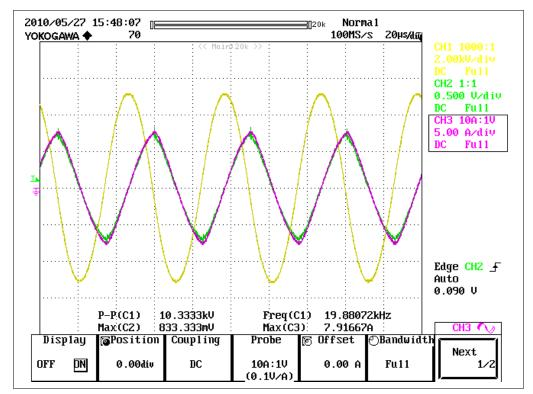
Ioad: 90pF CH1: output voltage CH2: current monitor 10V/A CH3: primary current cascade
