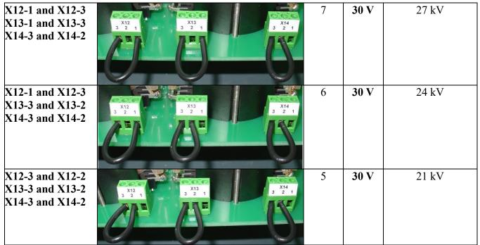
Remark: In an earlier version of this manual, the markings of pin 1 and pin 3 of X12, X13 and X14 were exchanged. Relevant for connection is however not the marking, but the position.
